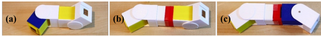
Fig. 3: (a) Two servo blocks connecting directly creates a relative rotation of 90-degree; (b) Extension block can be used to adjust the length of legs; (c) Rotation block can be used to adjust the rotation axis of legs.
